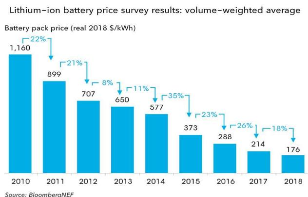
Figure 4: Li-ion battery pack price over time (volume-weighted average)<sup>10</sup>
