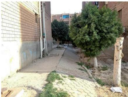
👎 Bad example of footpath: limited width and danegerous change of levels make walking unsafe.
