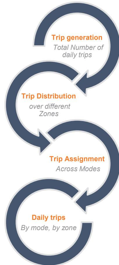
To conduct the quantitative side of the scenario analysis, indicators and variables were inputted together in a tabular spreadsheet. The spreadsheet contains a high-level and strongly simplified version of the **classical transport model**, which aims at predicting the total number of trips generated (Trip-Generation); a simplified distribution over space (Trip-Distribution); the choices of modes (Modal-Split); and the allocation of trips to modes (Trip-Assignment).
